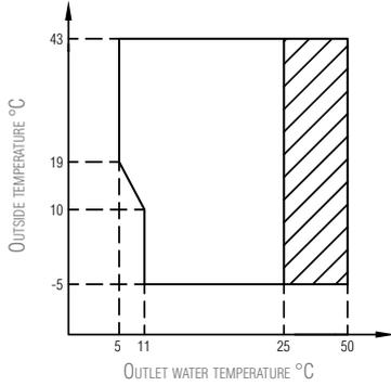
Operation range by heat pump with possible limitation and protection
