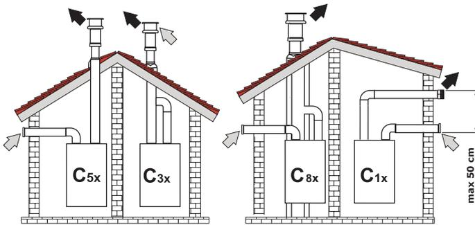
Fig. 3 - Example of connection with separate pipes
