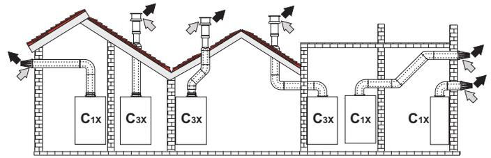
Fig. 2 - Example of connection with coaxial pipes
