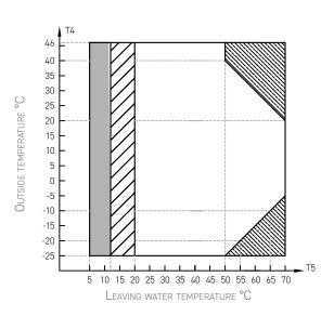
Operating range of heat pump with possible limitation and protection
