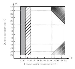
Operating range of heat pump with possible limitation and protection
