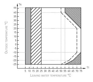
Operating range of heat pump with possible limitation and protection
